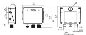
Structure and device dimensions, unit: mm (inch), decimal separator: period
