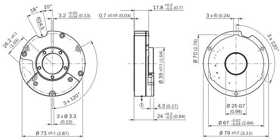
Measuring point for operating temperature
