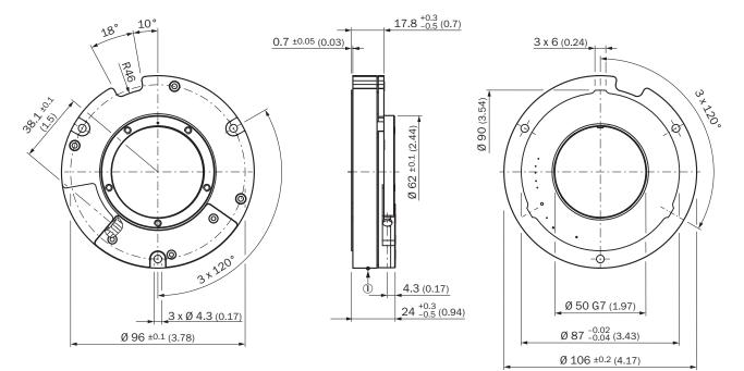
① Measuring point for operating temperature
