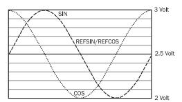
Signal diagram for clockwise rotation of the shaft looking in direction "A" (see dimensional drawing)1 period =  $360^{\circ}$ :  $1024^{\circ}$
