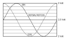
Signal diagram for clockwise rotation of the shaft looking in direction "A" (see dimensional drawing)1 period =  $360 \degree : 1024$
