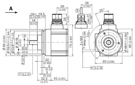
General tolerances according to ISO 2768-mk O R = min. bending radius 40 mm
