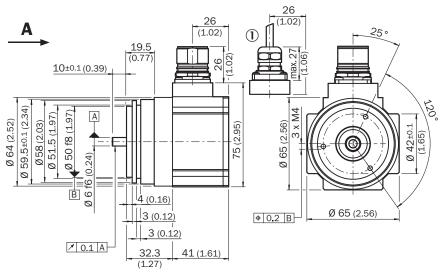
General tolerances according to DIN ISO 2768-mk R = min. bending radius 40 mm
