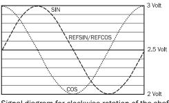
Signal diagram for clockwise rotation of the shaft looking in direction "A" (see dimensional drawing)1 period =  $360^{\circ}$ : 1024 Signal diagram for clockwise rotation of the shaft looking in direction "A" (see dimensional drawing)1 period =  $360^{\circ}$ : 1024
