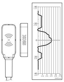
Assured switch on distance Sao 9 mm. Observe border areas for parallel approach: a minimum distance of 4 mm (typical) must be upheld when the actuator moves laterally to the sensor surface. This prevents early triggering due to the side preparation areas.
