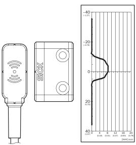
Safe switch on distance  $S_{ao}\,6\mbox{ mm}$
