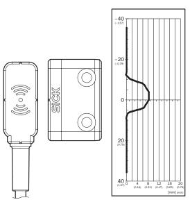
Safe switch on distance  $S_{ao}\,6\mbox{ mm}$
