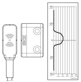
Safe switch on distance  $S_{ao}\ 6\ mm$
