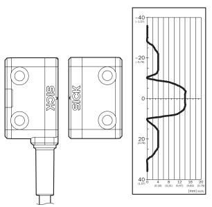
Assured switch on distance Sao 10 mm. Observe border areas for parallel approach: a minimum distance of 6 mm (typical) must be upheld when the actuator moves laterally to the sensor surface. This prevents early triggering due to the side preparation areas. "Standard" actuator, active side sensor surface
