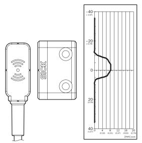
Safe switch on distance  $S_{ao}\ 6\ mm$
