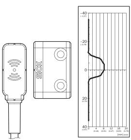
Safe switch on distance  $S_{ao}\,6\mbox{ mm}$
