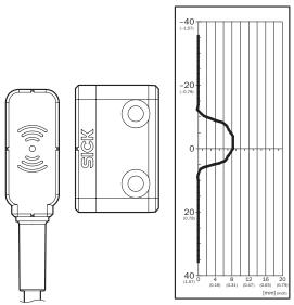
Safe switch on distance  $S_{ao}\,6\;\text{mm}$
