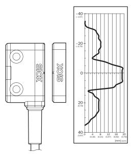
Assured switch on distance Sao 14 mm. Observe border areas for parallel approach: a minimum distance of 10 mm (typical) must be upheld when the actuator moves laterally to the sensor surface. This prevents early triggering due to the side preparation areas. "Standard" actuator, active front sensor surface
