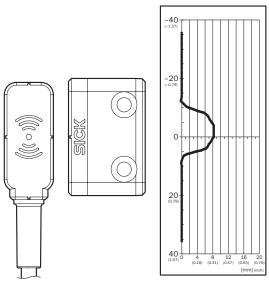
Safe switch on distance  $S_{ao}\,6\;\text{mm}$
