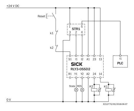
Parallel connection of two STR1 RFID safety switches to a Flexi Classic safety controller
