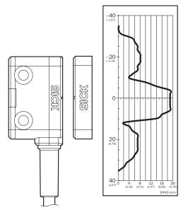
Assured switch on distance Sao 14 mm. Observe border areas for parallel approach: a minimum distance of 10 mm (typical) must be upheld when the actuator moves laterally to the sensor surface. This prevents early triggering due to the side preparation areas. "Standard" actuator, active front sensor surface
