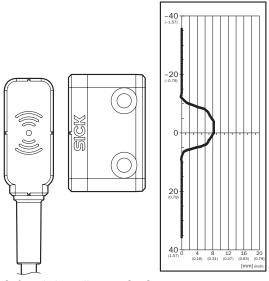
Safe switch on distance  $S_{ao}\,6~\text{mm}$
