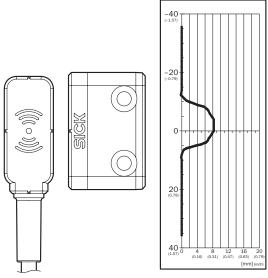
Safe switch on distance  $S_{\text{ao}}\,6\,\text{mm}$
