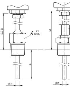
Dimensional drawing: housing, without process connection
