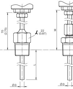
Dimensional drawing: housing, without process connection
