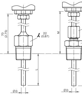
Dimensional drawing: housing, without process connection
