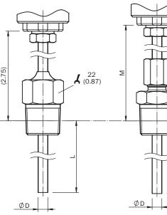
Dimensional drawing: housing, without process connection
