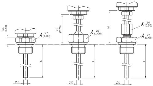
Dimensional drawing: conical threads
