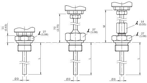
Dimensional drawing: conical threads
