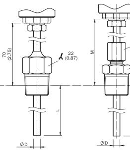
Dimensional drawing: housing, without process connection
