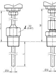
Dimensional drawing: housing, without process connection
