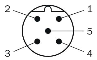
Connector M12, 5-pin, A-coded
