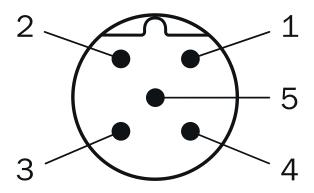
Connector M12, 5-pin, A-coded
