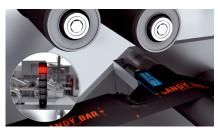
Continuous monitoring: the UFS constantly sends current process data via IO-Link, which can be used for automatic reporting of upset conditions and predictive maintenance planning.
