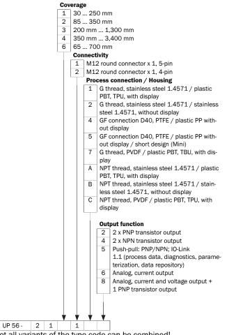
Not all variants of the type code can be combined! Dimensional drawing (Dimensions in mm (inch))
