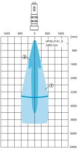
① Example object: aligned plate 500 mm x 500 mm
