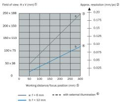
Take into account the following aspects when designing the application: the field of view geometry of the device, and the position of the field of view in the space in front of the device. Possible angles at which the objects can arise in relation to the device. For the planned working distance: resultant field of view length and width as well as the approximate resolution.
