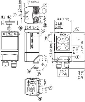
Structure and device dimensions, unit: mm (inch), decimal separator: period
