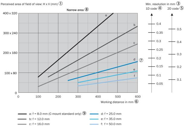
For S-mount and standard C-mount lenses, spacer rings are needed for working distances shorter than approximately 10 times the focal length. For compact C-mount lenses, spacer rings are not needed, but the built-in illumination cannot be used for distances shorter than 300 mm.
