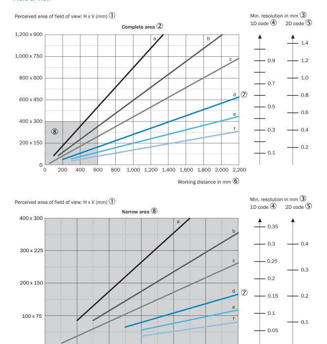
For S-mount and standard C-mount lenses, spacer rings are needed for working distances shorter than approximately 10 times the focal length. For compact C-mount lenses, spacer rings are not needed, but the built-in illumination cannot be used for distances shorter than 300 mm.
