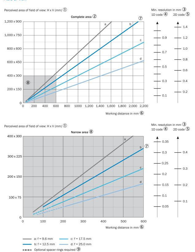
For S-mount and standard C-mount lenses, spacer rings are needed for working distances shorter than approximately 10 times the focal length. For compact C-mount lenses, spacer rings are not needed, but the built-in illumination cannot be used for distances shorter than 300 mm.
