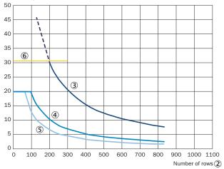
The maximum line rate is based on the number of sensor lines used
