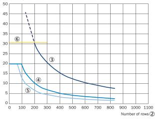
The maximum line rate is based on the number of sensor lines used ① Line rate (kHz)
