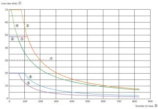
The maximum line rate is based on the number of sensor lines used
