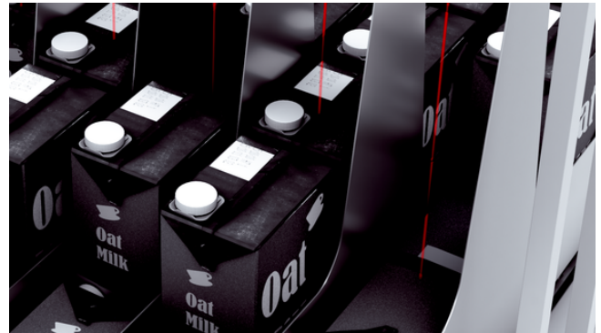
Using the “Two independent switching points” mode, standing and lying objects can be detected and distinguished from one another
