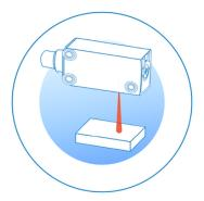
Thanks to foreground suppression, the sensors reliably detect very flat, poorly remitting, reflective, and uneven objects. Find out more in the video
