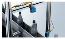
Base logic: User-definable logic functions with trigger sensors and switching signal delays
