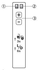
Function signal indicator (yellow), switching output
