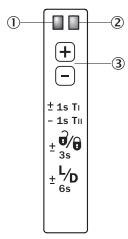
Function signal indicator (yellow), switching output
