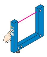
The yellow function indicator illuminates when the light received is at its optimum level. If necessary, increase sensitivity using the "+" button.
