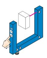
Yellow function indicator goes out. If necessary, reduce sensitivity using the "-" button.
