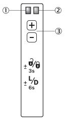
Function signal indicator (yellow), switching output
