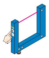
The yellow function indicator illuminates when the light received is at its optimum level. If necessary, increase sensitivity using the "+" button.
