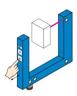
Yellow function indicator goes out. If necessary, reduce sensitivity using the "-" button.
