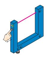
Press the teach-in button for 3 - 20 s. With the pushbutton pressed down, move several objects with carrier material (label objects to be detected) through the sensor. The yellow LED flashes at 3 Hz during the teach-in procedure. Recommendation: Move at least 3 objects through the sensor.
