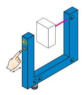
Release the teach-in button for < 20 s. If teach-in is suc-cessful, the function indicator (yellow LED) directly indicates the output state of the sensor. The switching threshold is now optimally set between background and object. The best possible operational safety is provided.
