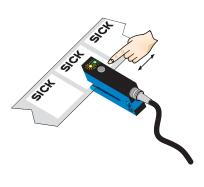
Release the teach-in button for <  $20 \, \text{s}$ . If teach-in is successful, the function indicator (yellow LED) directly indicates the output state of the sensor. The switching threshold is now optimally set between carrier and label. The best possible operational safety is provided.
