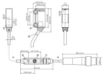
Length of cable: L1 = 155 mm, L2 = 156 mm
